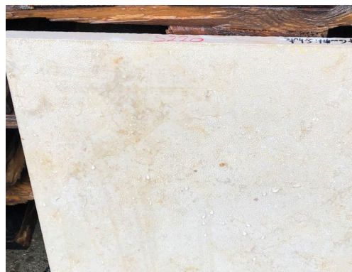
Figure 2: Slab (sandblasted) with AKEMI® Anti-Graffiti after cleaning with steam jet and AKEMI® Graffiti Remover
